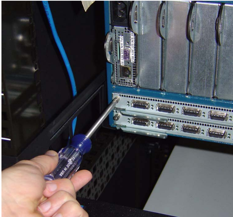
Figure 2-9: Securing Switch Card
